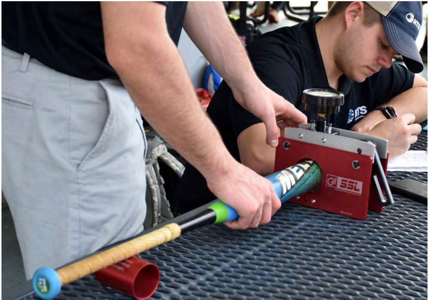
Two NTS bat lab experts/engineers, Marty Bindel & Jason Kelsch, performed compression testing on bats to gather data for a field test standard at the 2024 TOC.
